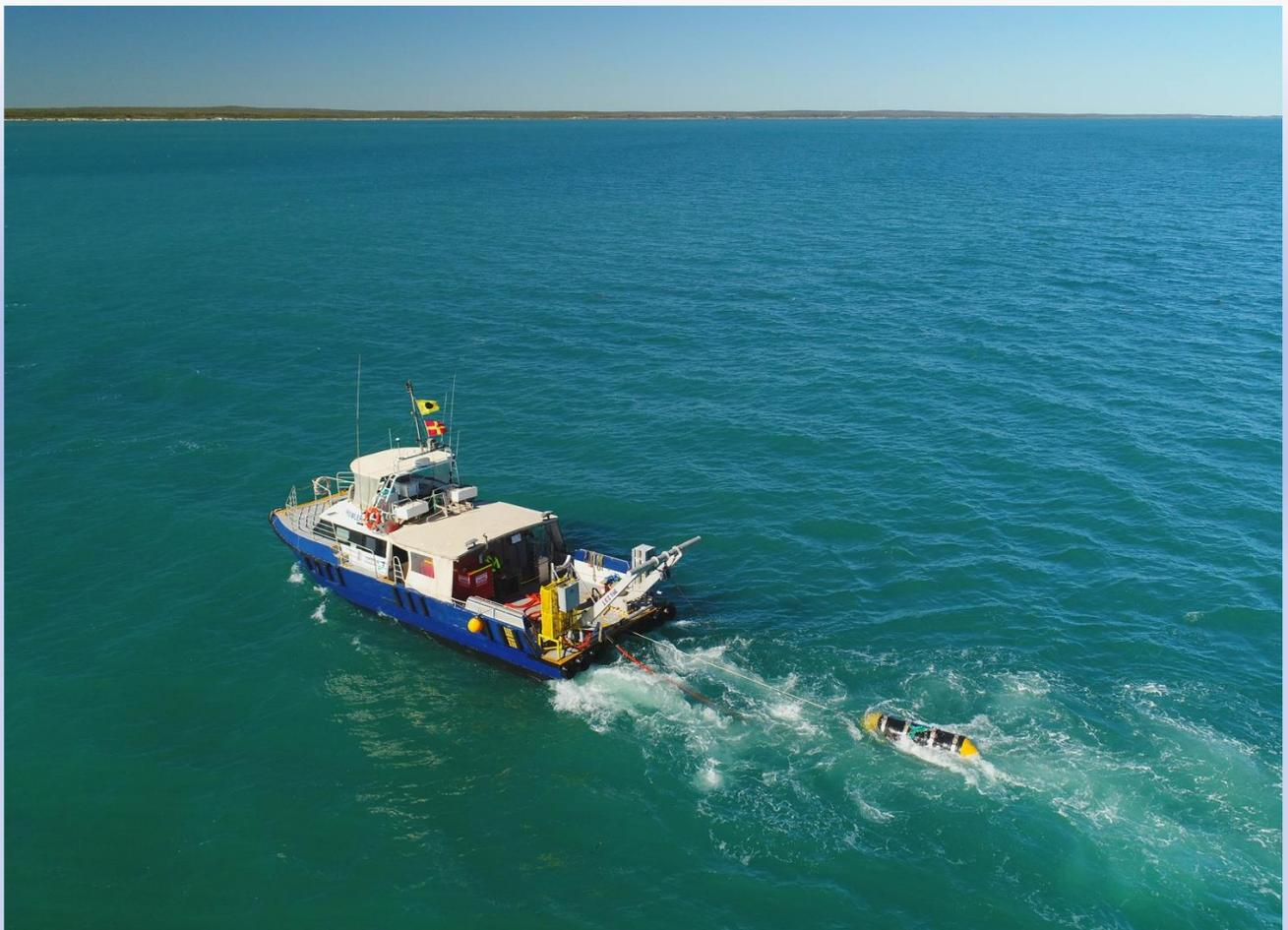
Image: The *Prowler* towing the airgun array during production operations
